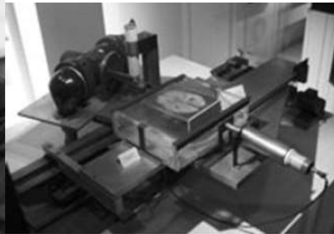
Laboratory scanner used by G.N. Hounsfield
